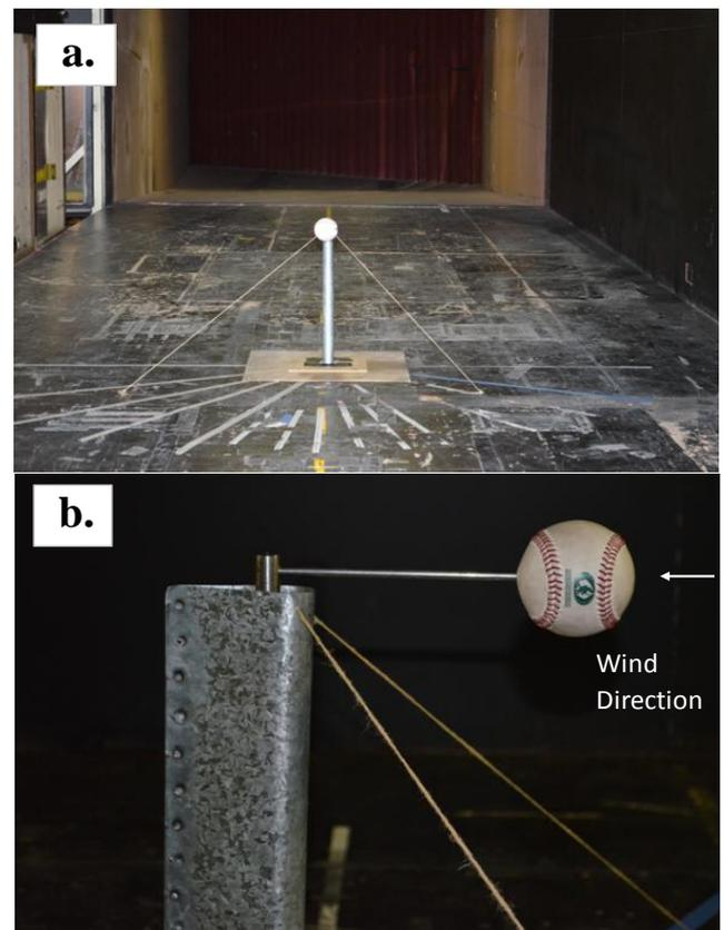
Figure 6. Experimental setup for wind tunnel testing of baseballs: (a) Front view and (b) Side view
