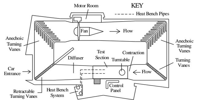
Figure 5. Plan view of RMIT Industrial Wind Tunnel
